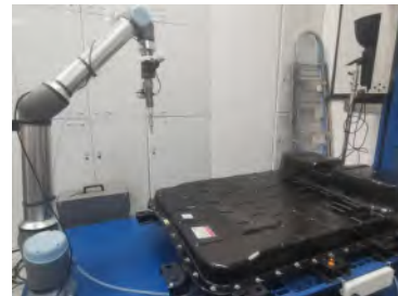
Fig. 5. Work platform equipped with robot arm
